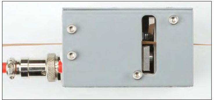
Side view of tab inserter showing cutter position.
